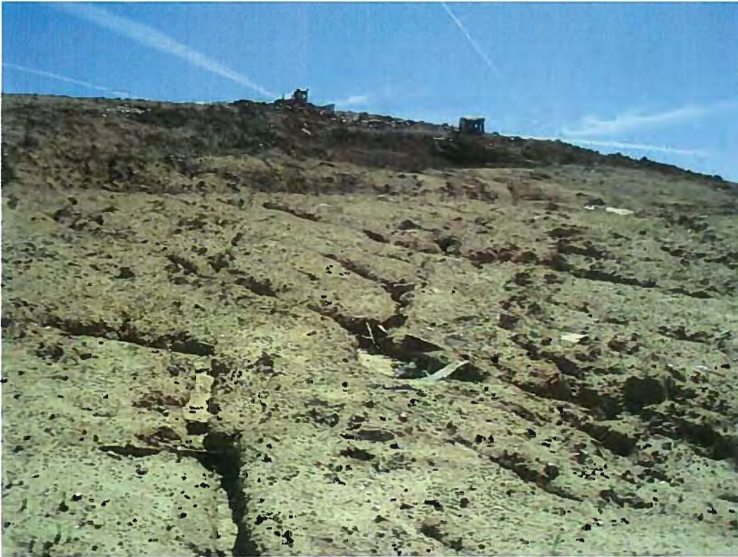
Date: 4/18/2012 Time: 11:48 A.M. Direction: southeast Photo by: S. Williams Exposure #: 009 Comments: erosion gullies & litter
